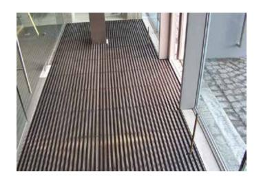
The foundation of TOPWELL 27mm SUPER mat are 27mm wide aluminium sections, connected by a stainless steel wire and separated by rubber rings, making it possible to roll the mat for better handling when cleaning. Brush strips are firmly inserted into the aluminium sections.
