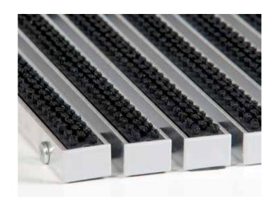
The foundation of TOPWELL 22 mm SUPER mats is 27 mm wide aluminium sections. which are connected by a stainless steel wire and separated by rubber rings, making it possible to roll the mat for better handling when cleaning.
