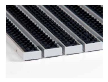
The foundation of TOPWELL 17mm SUPER mat are 27mm wide aluminium sections, connected by a stainless steel wire and separated by rubber rings, making it possible to roll the mat for better handling when cleaning. Brush strips are firmly inserted into the aluminium sections.
